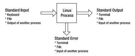
Figure 2-2. The process input and output data streams
