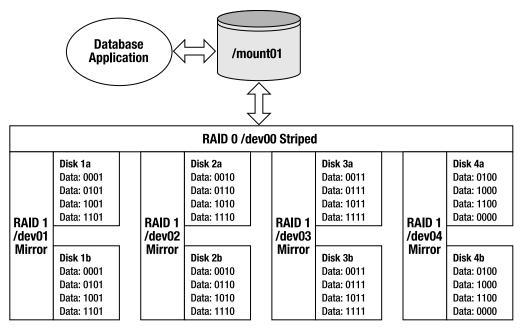
Figure A-8. A RAID 1+0 mirrored and then striped device
