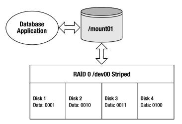
Figure A-2. A four-disk RAID 0 striped device
