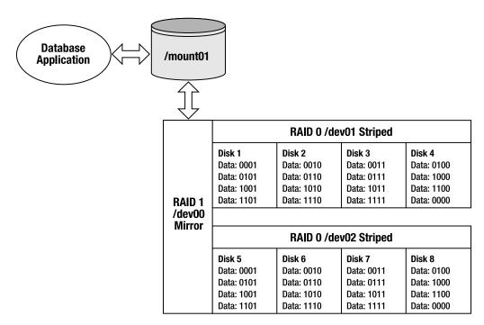
Figure A-7. A RAID 0+1 striped and then mirrored device
